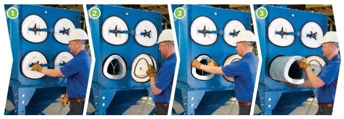
Loosen cover with 4-lobe knob. Knob has center lug enabling power tool operation.
